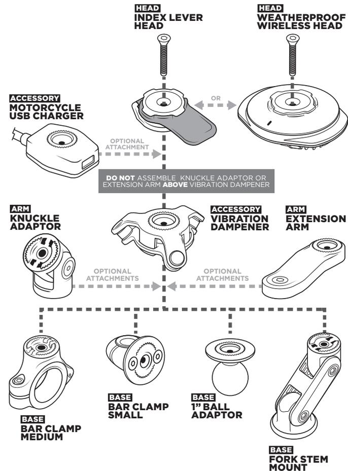
**DO NOT ASSEMBLE KNUCKLE ADAPTOR OR EXTENSION ARM ABOVE VIBRATION DAMPENER**
